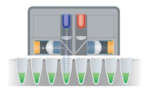
As the CFX Opus Systems' optics shuttle travels across the plate, light is focused into the center of each sample well. Side view of the optics shuttle shows the 450-490 nm LED firing and SYBR® Green emitting at 520 nm into the detector.
